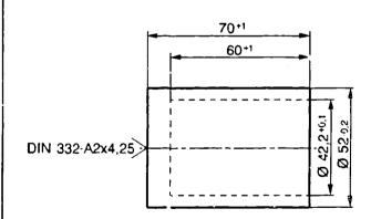
Tool for pressing deep-groove ball bearing onto intermediate bearing:
